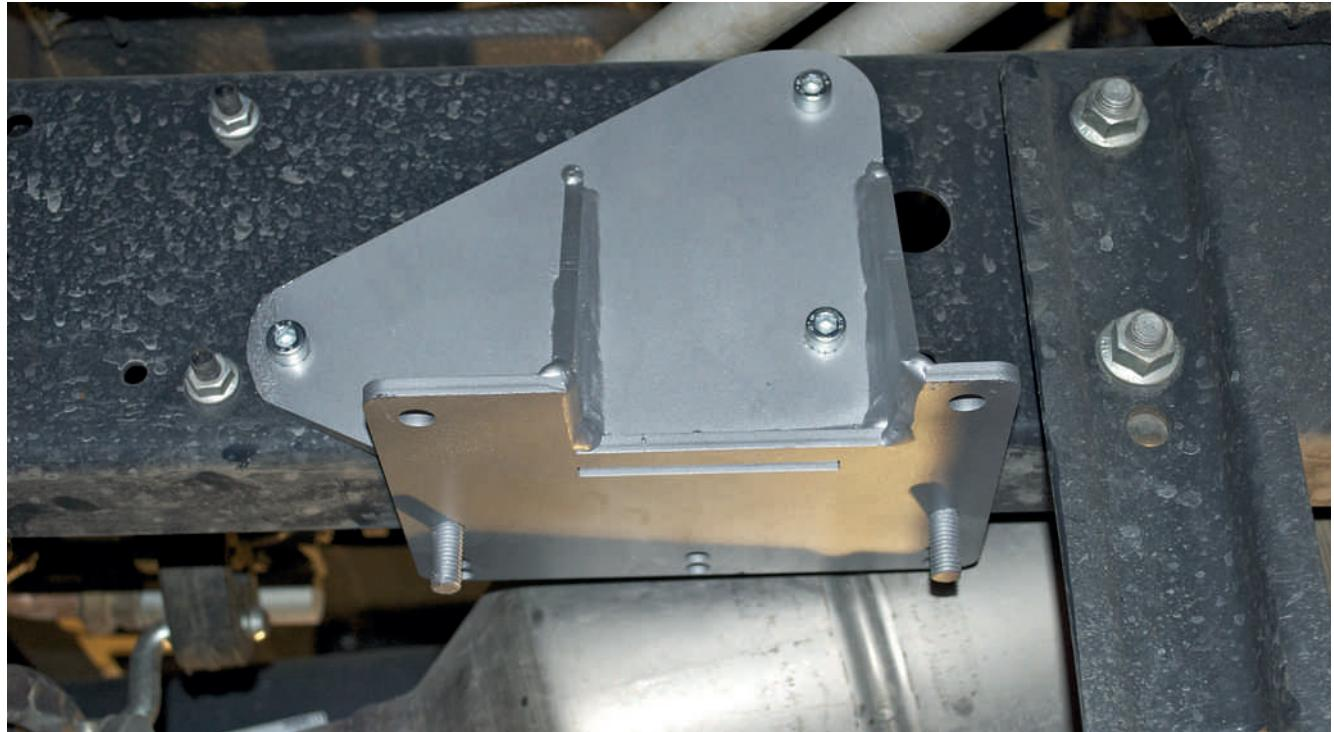
The adapter must be placed just behind the gearbox cradle, follow the same procedure as for the front left adapter.
