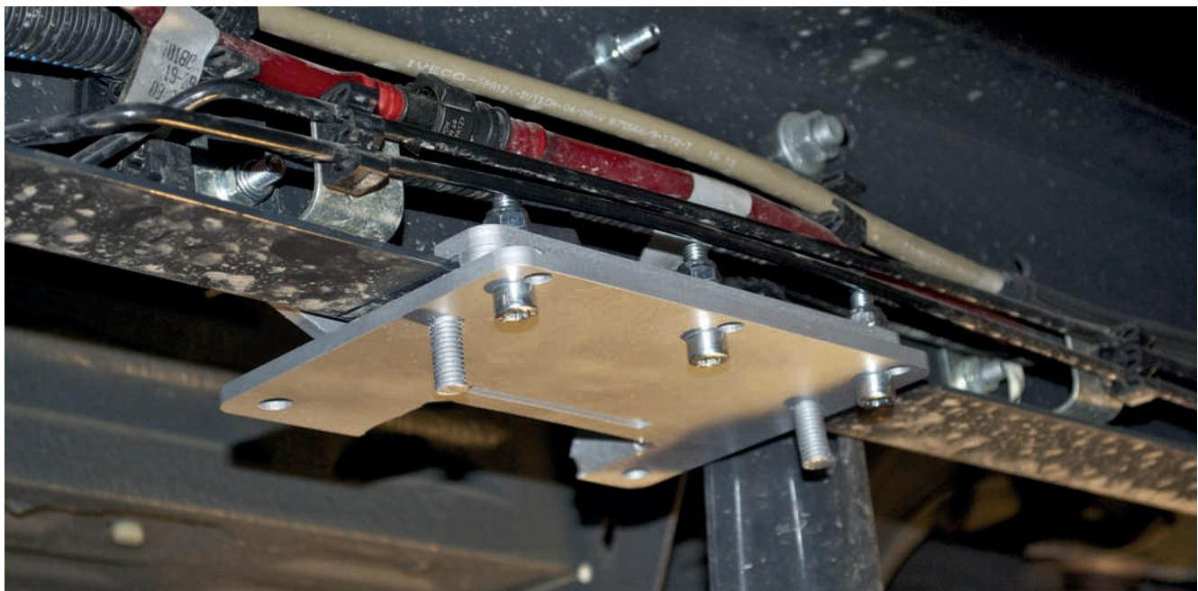
Insert the sealing plate in the hole on the frame, put the adapter and push towards the front. Then mount the clamp on the inside of the frame.
