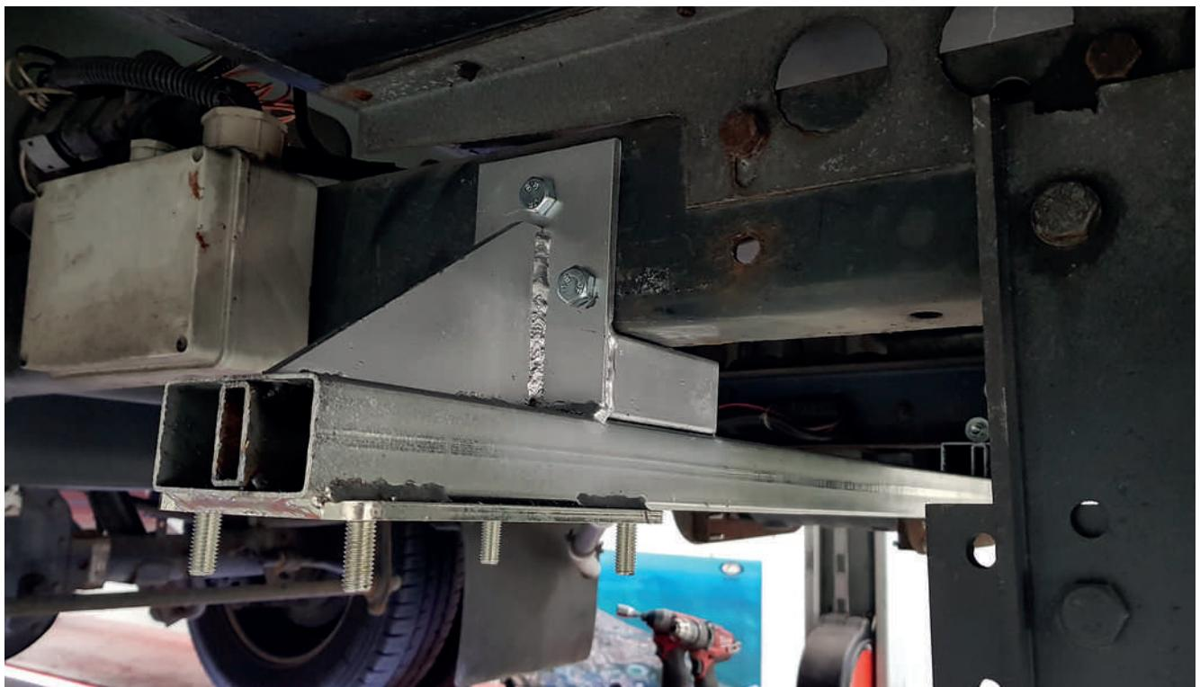
Put the adapter behind the rear axle. Drill the holes only after the adapter is completely inserted. In some cases it's possible to use holes already present on the chassis.
